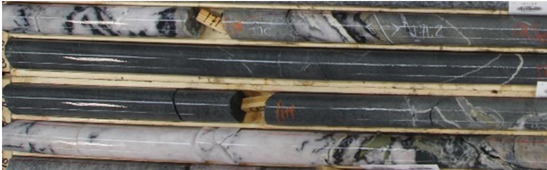
Figure 7-14: Mineralized Veins in Diorite Dyke
