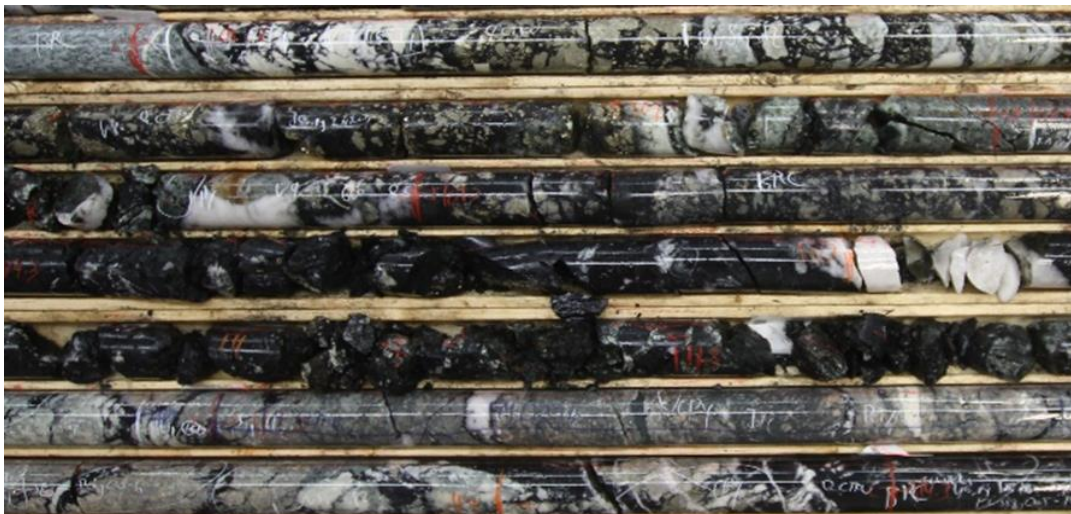
Figure 7-13: High-Grade Quartz-Tourmaline-Carbonates-Pyrite Hydrothermal Breccia in Creek Zone
