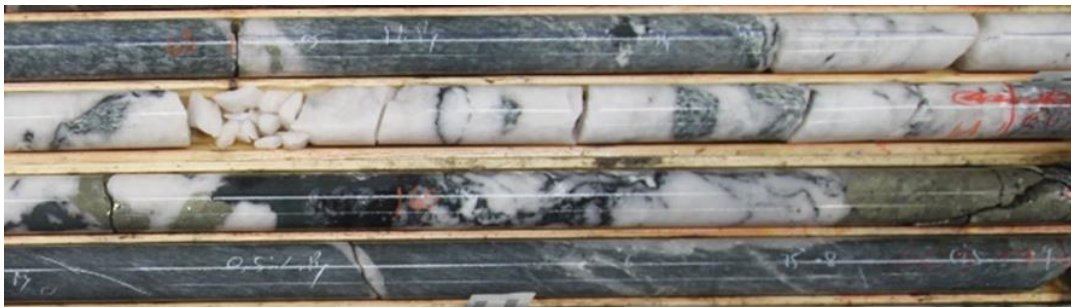
Figure 7-12: High-Grade Decimetric Pyrite Blebby Masses in Quartz-Tourmaline-Carbonates Veins in Creek Zone
