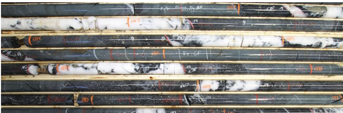
Notes: Extension of Main Dyke L.C. Beliveau at depth from the New Beliveau deposit showing quartz-tourmaline-carbonates veins with coarse pyrite and tourmaline-silica-carbonates alteration (PC-17-197, 681-692.5m, 5.49 g/t Au over 8.46 m between 682.19-690.65 m). Source: Probe Metals, 2021.
