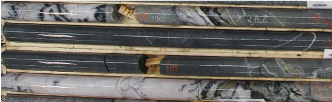
Figure 23 - Mineralized veins in diorite dyke (CO-18-39, 0.35 g/t Au over 3.00m between 173.00-176.00m)
