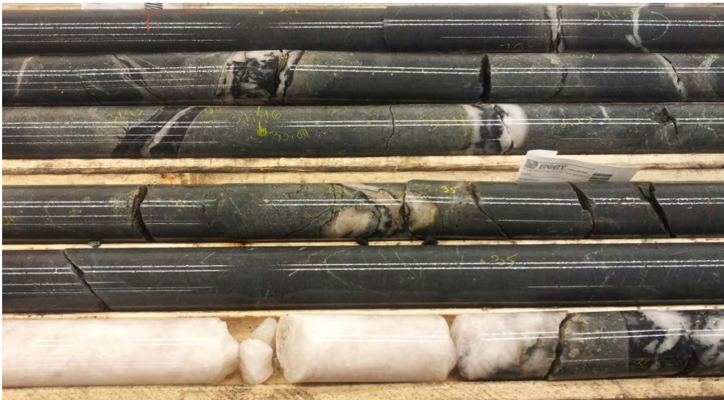
Figure 31 - Quartz-carbonate-tourmaline tension veins with silica and sericite alteration and 1-2% pyrite in a dacitic unit (LP-11-27, interval between 29-36m showing part of an intercept of 2.84 g/t Au over 53.6m)
