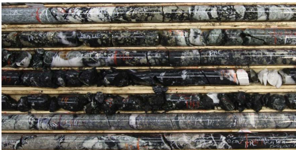
Figure 22 - High grade quartz-tourmaline-carbonates-pyrite hydrothermal breccia in Creek zone (CO-18-64, 9.6 g/t Au over 9.1m between 105.00-111.00m)
