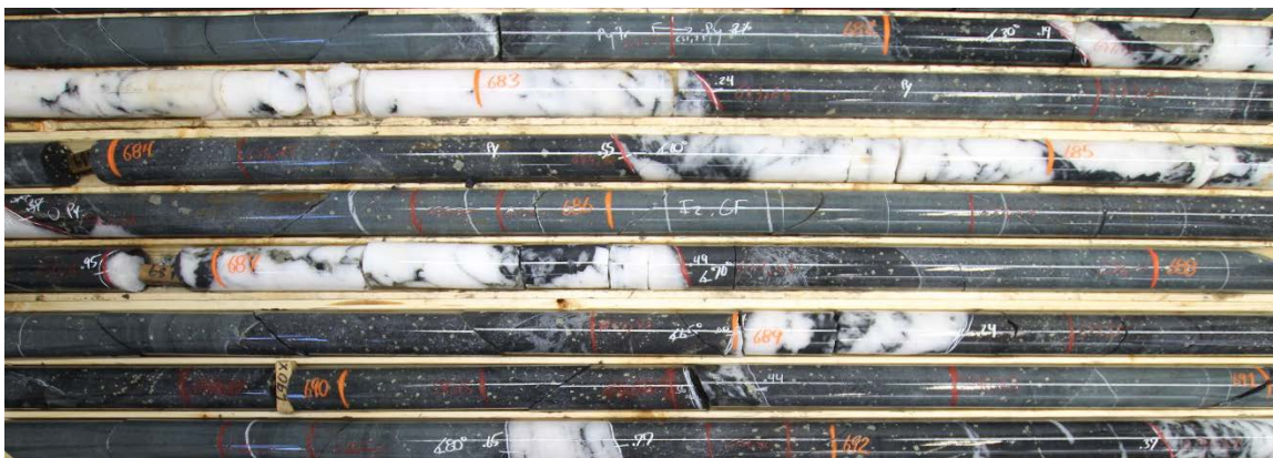
Figure 16 - Example of Dyke zone (extension of Main Dyke L.C. Beliveau at depth) from the New Beliveau deposit showing quartz-tourmaline-carbonates veins with coarse pyrite and tourmaline-silica-carbonates alteration (PC-17-197, 681-692.5m, 5.49 g/t Au over 8.46m between 682.19-690.65m)
