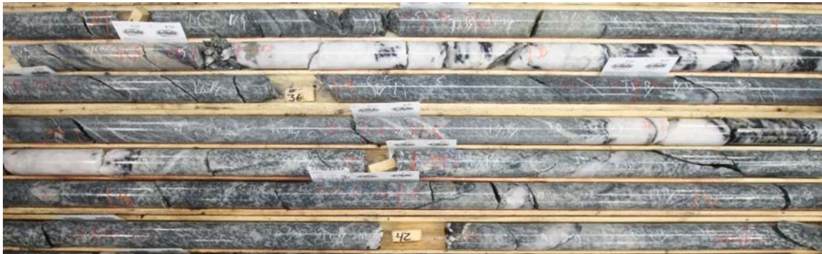
Figure 20 - Typical Courvan mineralized zone showing quartz-tourmaline-carbonates veins with coarse and silica-sericite-K feldspars-carbonates alteration in Bussiere zone (CO-18-31, 5.08 g/t Au over 8.00m entre 33.50-41.50m)
