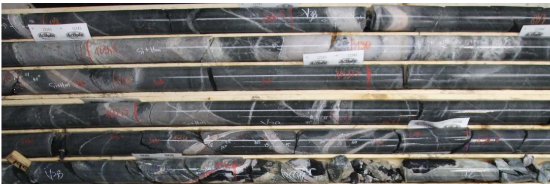
Figure 26 : M zone in basalts (MO-19-16, part of an interval grading 5.9 g/t Au over 11.5m between 184.00-195.50m)
