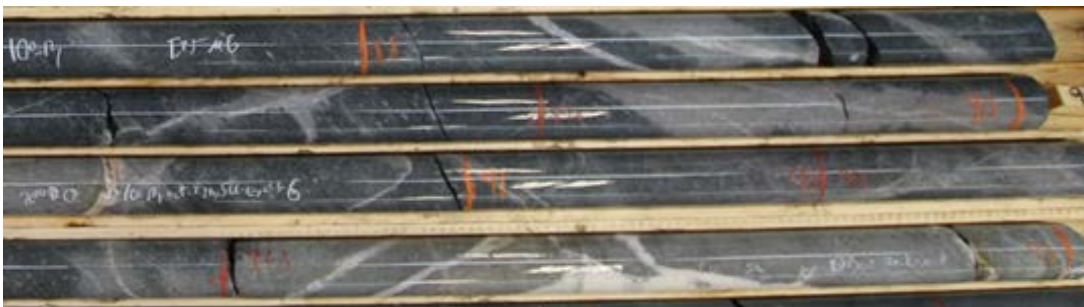
Figure 29 : P zone in a diorite dyke (MO-20-53, 2.4 g/t Au over 5.70m between 87.60-93.30m)
