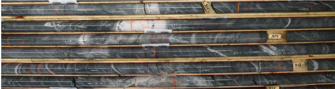
Figure 17 - Example of Volcanic zone from the North deposit showing quartz-tourmaline-carbonates veins with pyrite and silica-sericite-carbonates alteration hosted in mafic volcanoclastic rocks, namely agglomerates (PC-18-328, 4.25 g/t Au over 8.70m between 305.30-314.00m)
